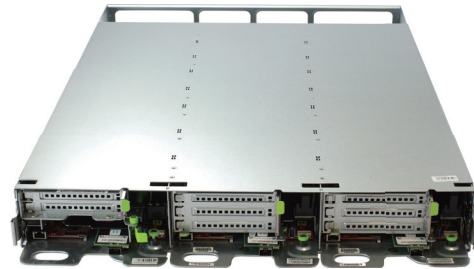
Three Wiwynn SV7220G3 servers in a 2OU (Open Rack) space
